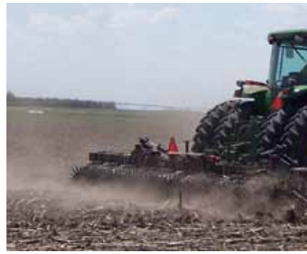
Rotary hoes can be operated at high speeds of 7 to 10 miles per hour.
