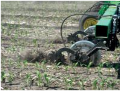
Single-disc injection coulters have low disturbance and can be operated at higher speeds.
