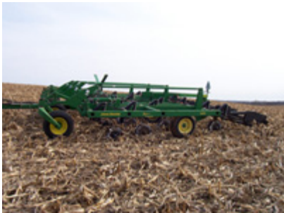
Adding vertical tillage attachments to an old chisel plow frame results in a versatile tool that can eliminate compaction.
