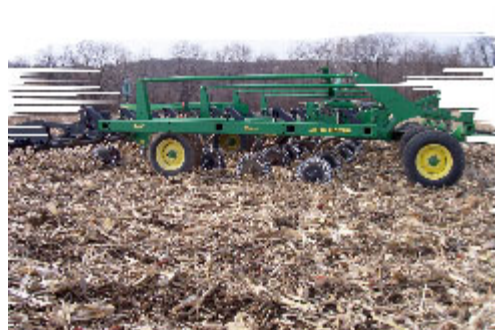
Shallow vertical tillage done with wavy coulters is an effective way to size and incorporate residue which aids decomposition over winter without risking high levels of compaction.
