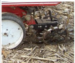
Spike closing wheels fracture the soil and aid with effective seed trench closing.
