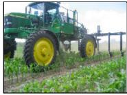
John Deere self-propelled sprayers, equipped with liquid fertilizer toolbars, offer a greater window for side-dress application
