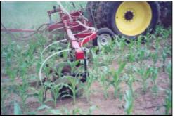
Adding a coulter and spring mounted injector to existing toolbars is an easy and cost effective way to create a side-dressing toolbar.
