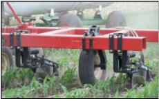
Existing toolbars can be retrofitted with anhydrous coulters for high-speed application as well.
