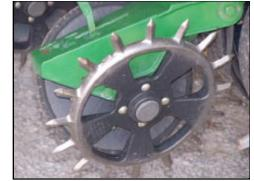
Spike closing wheels have proven to be invaluable in some planting conditions, creating very good seed-to-soil contact in less-than-ideal conditions.
