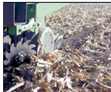
Heavy piles of residue make proper planter performance more difficult.
