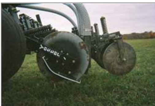
Angled blades with sealing discs provide no-till farmers a manure application option not available in the past.
