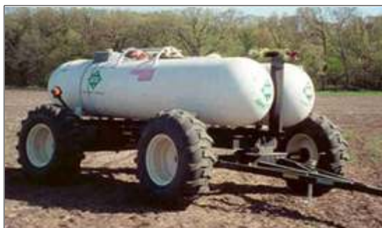
New NH 3 wagons have increased capacity while lowering compaction.
