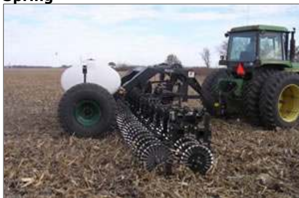
Vertical tillage machines can be used in the fall to size Bt cornstalks to encourage residue breakdown.
