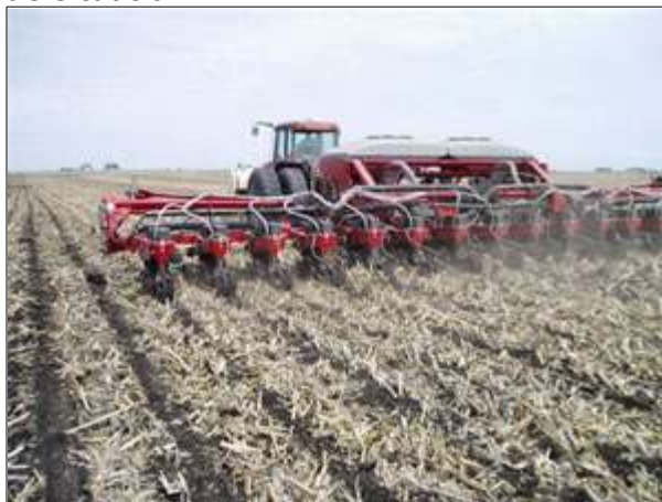
Planters need to be properly equipped to handle multiple years of heavy residue as Bt cornstalks often do not breakdown in one year.
