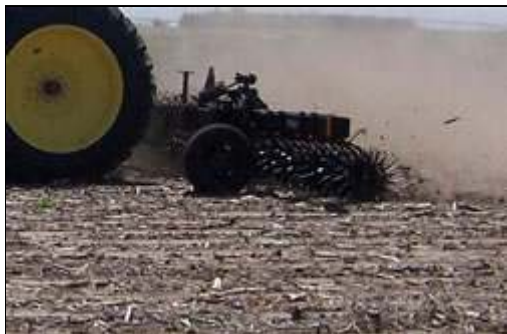
Rotary hoeing aerates the soil aiding earlier planting in no-till.
