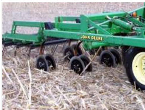
Vertical tillage sizes residue earlier to promote residue breakdown and soil warm up.
