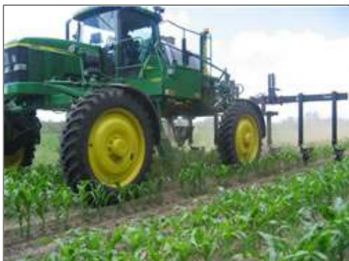
Self-propelled side dressing machines increase application windows with greater ground clearance and faster speeds.
