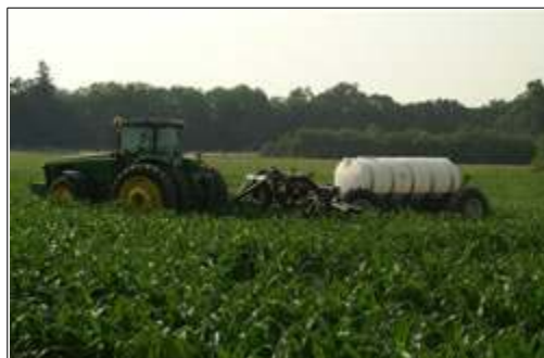
New equipment such as auto-guidance and all-wheel-steer carts make side dressing easier than ever before.
