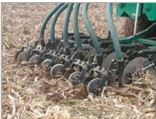
Avenger® coulters running in corn stalks with smooth sealing discs
