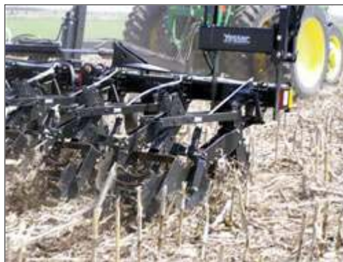
Coulter, residue manager, knife and rolling basket to make the perfect seedbed
