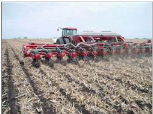
Planting in high residue conditions with Sharktooth® Wheels.
