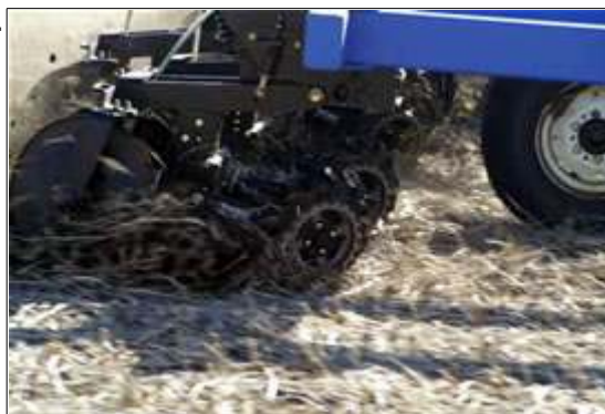
Residue managers clear residue ahead of berm builders.
