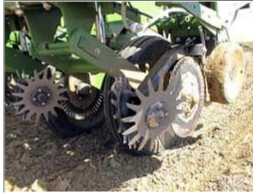
Unit mount fertilizer coulters with optional Residue Manager
