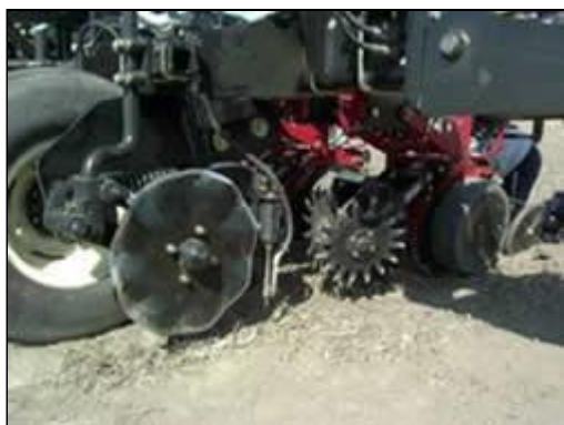
Fertilizer coultter with Coulter and Residue Manager combination
