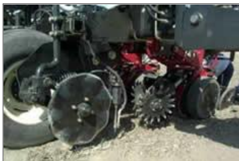
2995 Fertilizer coulters with liquid injection tube
