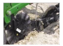
If this process of adjusting the fertilizer coulter is neglected, there is increased potential for crop damage. If fertilizer is not properly distributed, it may have an excess of product too close to plant roots, causing burning and destruction resulting in lower yields. Again, the labor time involved in the maintenance of your coulter for proper placement is a small price to pay when one considers the potentially devastating yield loss that could result from not doing so.
