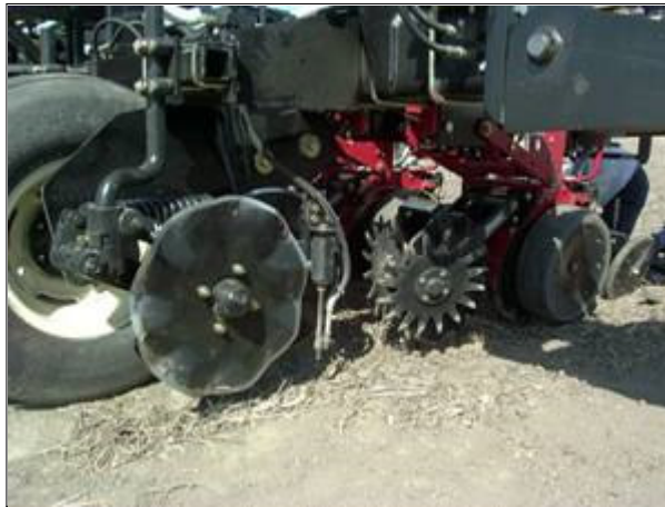
Coulter tillage with injection fertilizer placement and residue management
