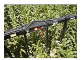
Fertilizer is injected using the same delivery system and controller for the spray boom. Fertilizer coulters slice open the soil and an injector rod keeps open the slot for a brief moment so fertilizer can be injected. By the very nature of its design, this application process can be done at high ground speeds while leaving the surrounding soil surface virtually undisturbed.
