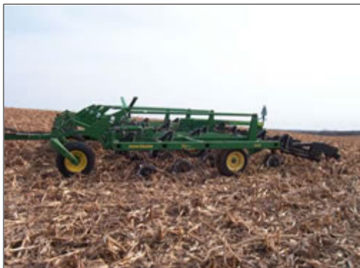
Vertical Tillage Attachment on JD 2400
