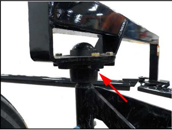
Grease pivot joints annually.
