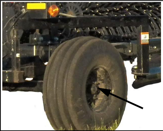
Grease main wheel bearing annually.
