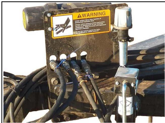
Wiring Harness and Hoses in Storage Position
