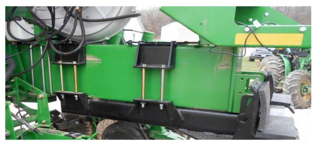
STEP 3: Insert the lock pin, 9010-374 5/8" X 10 ½" (JD planters), 9010-375 1" X 10 ½", (CHN planters), & 9010-376 1 ¼" X 13 7/16" (Kinze planters), through the frame anchor slotted holes. Install washers & roll pins on each end.
