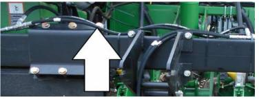
**STEP 8:** Install 1) 2515-435 -6 / -6 / -8 Tee to connect the pressure hoses from step 7. Install 1) 2515-435 Tee to connect the return hoses from step 7.
