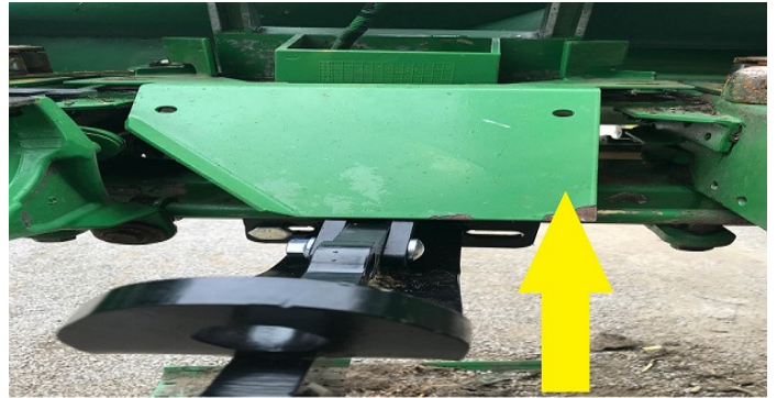
MOUNTING BRACKET ASSEMBLY INSTRUCTIONS (ROW 2-3 AND 10-11) JD 1293 (12 ROW) CORN HEAD (ONLY)
