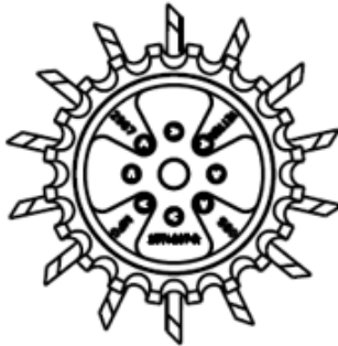
BEVEL WHEEL ASSEMBLY W/FLOATER WHEEL RIGHT HAND 2966-140-BW-FW(SHOWN) LEFT HAND 2966-141-BW-FW
