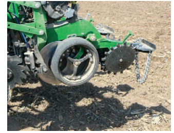
The Twister's rounded center ring maintains consistent depth.
