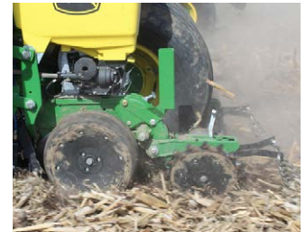
The Twister fractures the sidewall as it rolls through the field.
