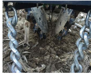
The Twister crumbles soil to break up sidewall compaction and eliminate air pockets.
