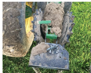
The Twister's rounded center design prevents mud buildup.
