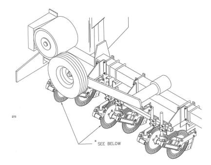
\*Note - Before transporting, two of the coulters must be pivoted to clear the endwise transport wheel
